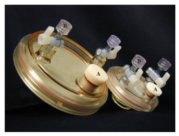
Figure 2: 50 & 10 ml Disposable Vessels Fill Port - A; Syringe Ports - B
