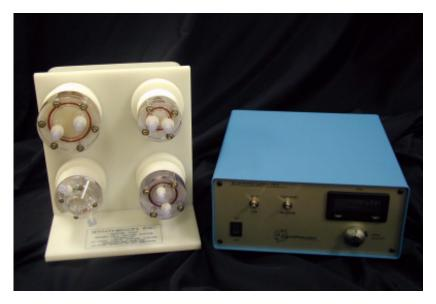
Figure 1: RCCS-4SC Rotator Base, Vessels & Power Supply
